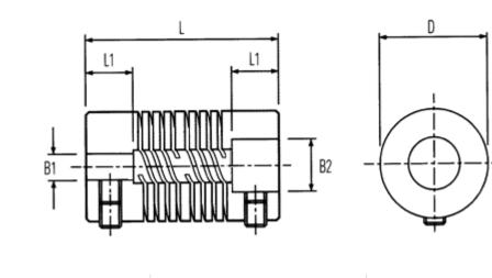
B1: Pre-drilled= 3.0B2: Pre-drilled= 6.00D= 15.9L= 25.4L1= 6.5Max angular displacement= 0.20Max B1 & B2= 8.00Max parallel displacement= 5
